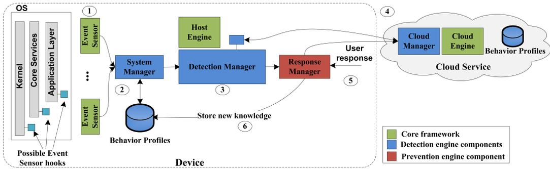
Figure 1: Proposed cross-layer IDS framework for mobile platforms.
